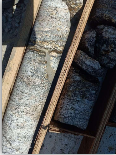
Figure 9: Grouting seen while drilling
