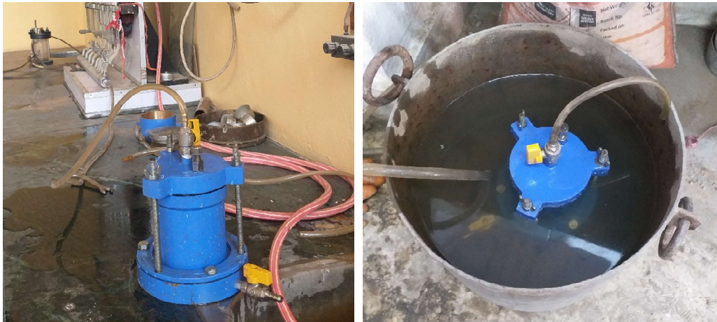
Figure 3.1 Constant Head Permeameter and Constant Head permeameter placed in sink
