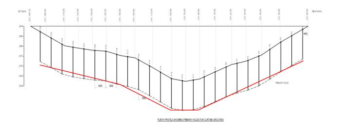
In above picture dotted plinth profile is as per actual construction and red line is according to desirable profile.
