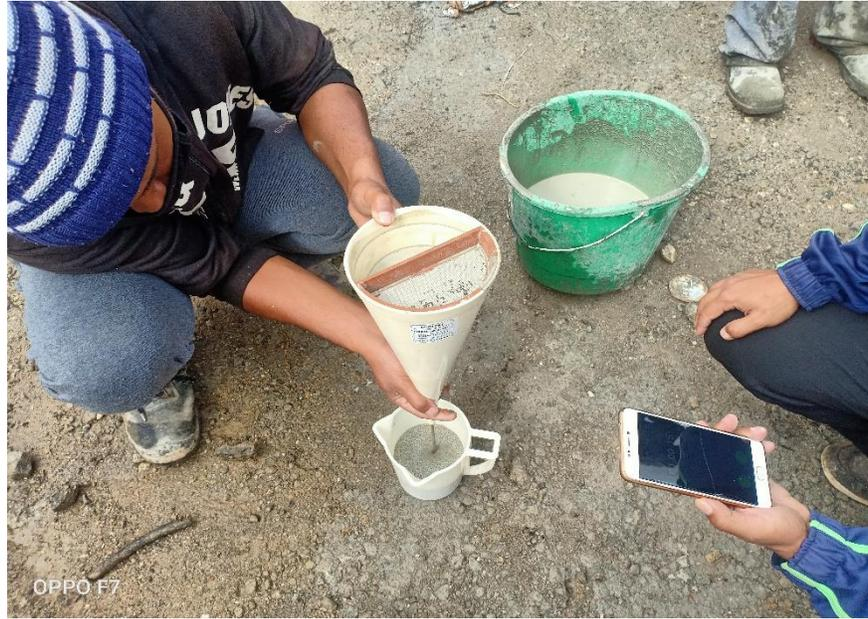
Fig: Marsh cone flow test of grout
