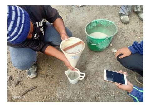
Fig: Marsh cone flow test of grout
